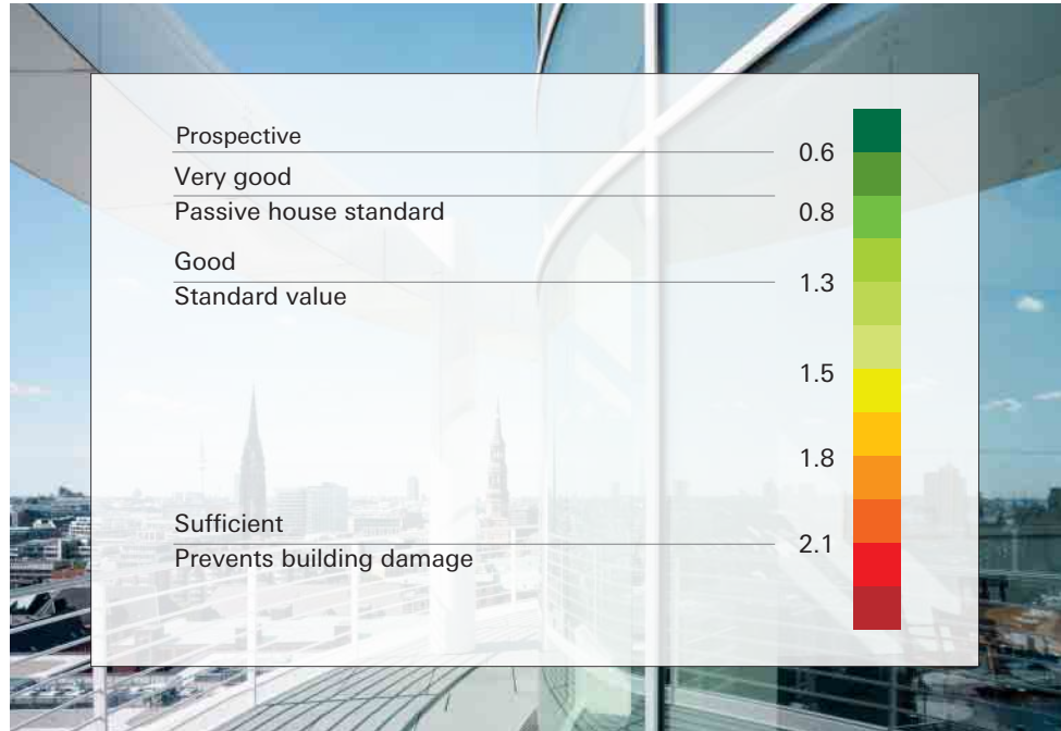
Graphic to 1. & 2.: Heat transfer coefficient [(W/(m 2 *K))] Characteristic values for the heat transfer coefficient U_w of the entire window or U_{CW} value of the façade, taking into consideration the U_f and U_g values.
